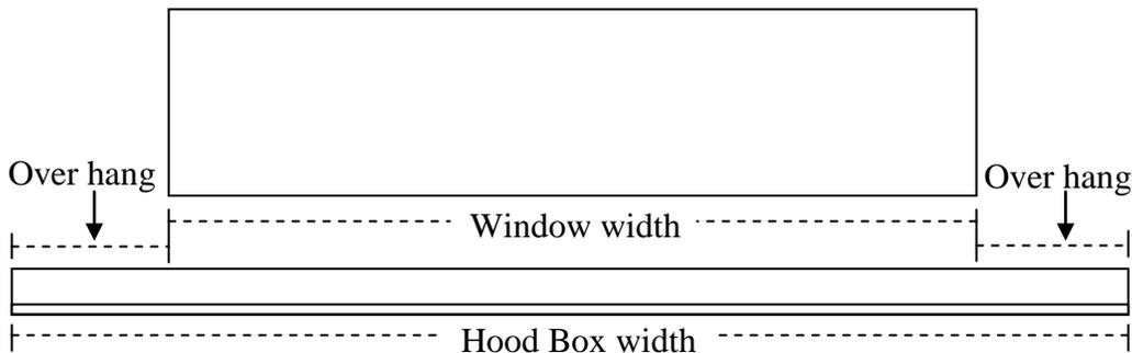
The left hand screw for the Hood Box should be placed to the left of the top corner of the window at the attachment point of the over hang and 180mm higher (the height of the Hood Box). If installing on a brick wall NEVER put the screw into a mortar line. If the position you need to drill is over a mortar line move up to the bottom of the brick above that position.
